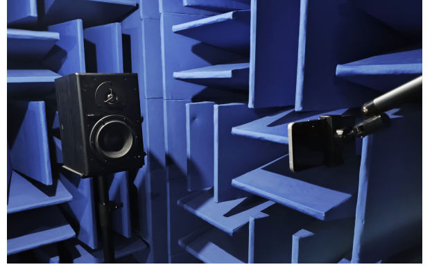
Fig. 7. The acoustic system utilized for measuring the impulse responses of the SPMA
