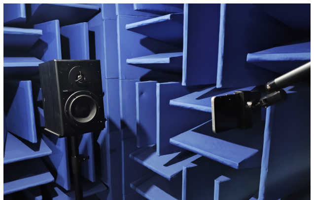
Fig. 2: The acoustic system utilized for measuring the impulse responses of the SPMA.
